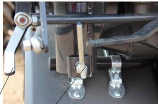
**Fig. 17** The locks on the sideboards of the body.
